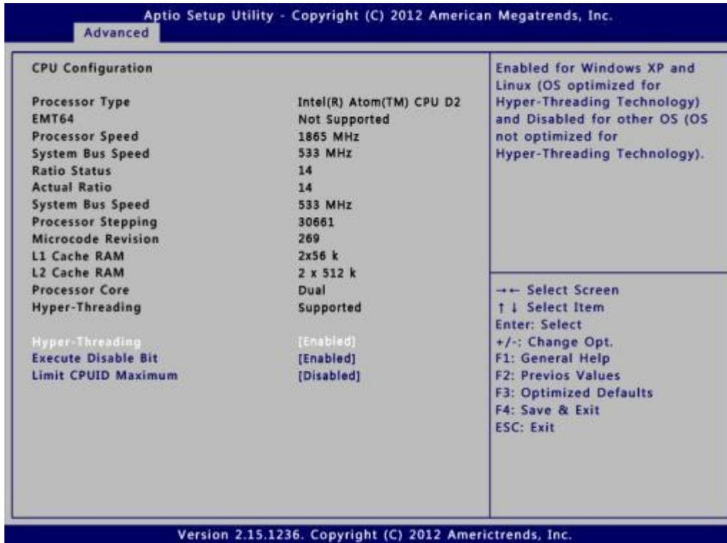
**Hyper-threading:** Enabled for Windows XP and Linux (OS optimized for Hyper-Threading Technology) and Disabled for other OS (OS not optimized for Hyper-Threading Technology). When disabled, only one thread per enabled core is enabled.
