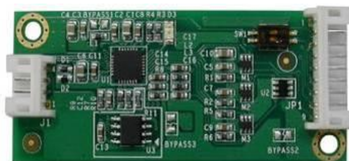
Figure 5.1: Bird's Eye View of Control Board
